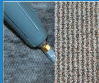
Tip orientation for proper edge sealing - excess glue is directed onto the back
