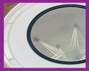
Fill the cleaning bucket with water so the upper ring of bristles is about 1-2 cm covered with water. Insert the tool to be cleaned vertically and with slow, circular stirring movements until a sufficient cleaning effect has been achieved.
