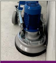
The grinding head can be adjusted with a clever locking system in both directions.
