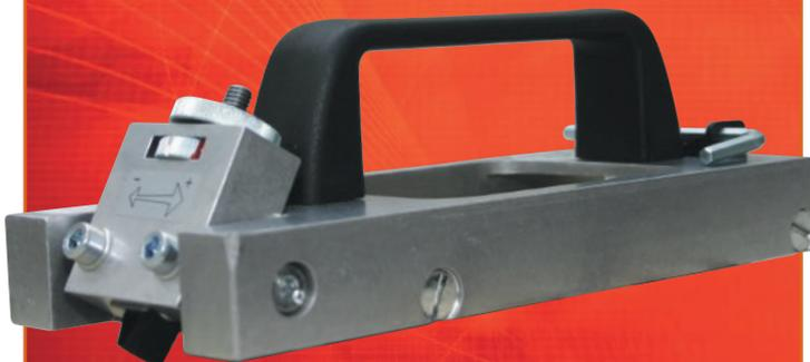
The wheeled Super Groover is a box groover ideal for small and medium areas. It also works well on safety floorings. The blade is adjustable in height to enable uniform grooving at various depths.
