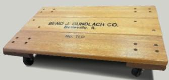
This dolly is made from solid 3/4" hardwood and has a lacquered finish. Has four ball bearing swivel casters with 2" diameter polypropylene wheels. Can also hold miscellaneous equipment and adhesive buckets. Measures 12" wide x 20" long x 4" high. Dolly has a 600lb capacity. Weighs about 9 1/2 lbs.
